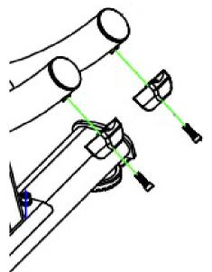
The Rail Bumpers mount points do not allow for easy removal off the back of the machine for the units listed above. You will need to remove the bolts holding the upper rail mount to the front frame and the rail support bar from it's mounting point as well. Once the front frame is free of the rail assembly the carriage will slide cleanly off the top of the rails and can be maneuvered on easily on it's own.
