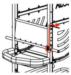
Note: The green reset button will be anchored to the mount plate that screws into the front of the unit. It can be removed by unscrewing the small locking bolt off the back of the plate and then pressing the button itself through the plate.
