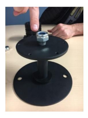
5. Install M16 nut on top of upper plate and secure with an Adjustable Crescent Wrench or metric 16 wrench. This will prevent bumper from getting loose in the future.
