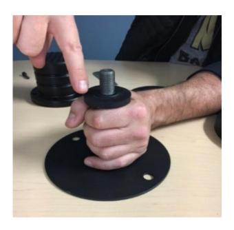
3. Insert new foot through the frame of the TireFlip and put rubber washer on top flat side DOWN. (photo does not show TireFlip frame)
