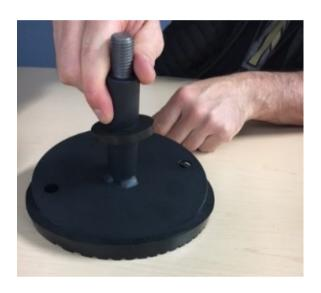
1. Remove rubber cover from the old foot and install on new foot.
